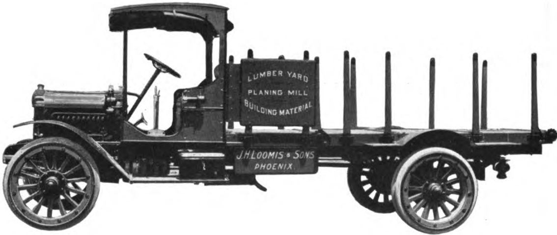
BROCKWAY MODEL "K" TWO-TON WORM DRIVE LUMBER TRUCK Manufactured by Brockway Motor Truck Co., Cortland, N. Y.
